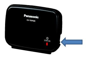
3. Plug the AC adaptor of the repeater to an electrical outlet.
