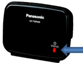
2. On the desk phone, press and hold **OK** until the display shows “Please Wait...”. The registration is complete when the display shows “Registered”.
