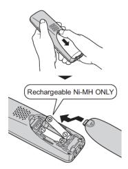
**2.** Remove the plastic wrapper from the rechargeable batteries included in the box, and place them into the handset.
