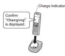
**3.** Place the handset into the charger and confirm that "Charging" is displayed. Charging the unit takes about 6 hours. When the batteries are fully charged, the charge indicator goes off and "Fully charged" is displayed. You are now ready to make and receive calls from the cordless handset.
