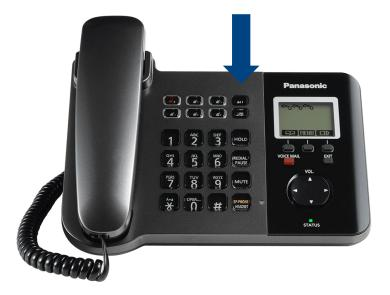
2. Press and hold the **ALL** button on the base unit for about 4 seconds until the status indicator flashes **red**. The base unit will emit a beeping sound.
